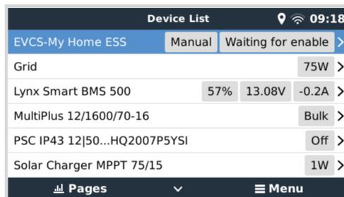
Highlight the EVCS then press spacebar or cursor right to enter the next menu and at the setup menu item press spacebar again to enter the setup menu. See the [EV Charging Station setup \[13\]](#) and the [Description \[2\]](#) chapter for the meaning of the available options.
