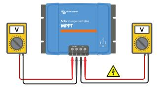
3. Compare both voltages, the PV voltage needs to be 5V higher than the battery voltage for charging to commence.
