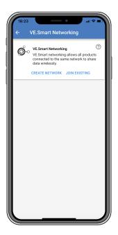
The VE.Smart network allows a variety of products connected to the same network to share data via Bluetooth. The VE.Smart network is especially designed for smaller systems that do not have a GX device installed.
