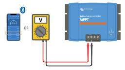
2. Use a multi meter to measure the voltage at the battery terminals.
