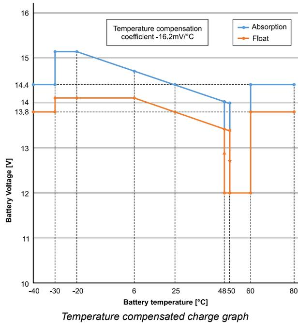
By default, the solar charger uses its internal temperature for battery temperature compensated charging. An internal temperature reading is taken in the morning and then again when the solar charger has been idle for at least one hour, for example when the charger is not actively charging a battery or supplying a load.
