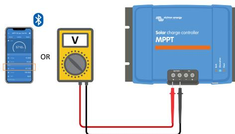
2. Measure the battery voltage on the terminals of the battery using a multi meter.
