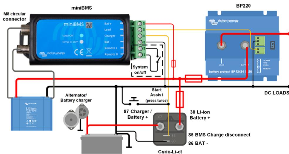
Figure 2: Application example for a vehicle or boat, with system on/off switch between H and L
